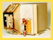
is the energetic particle spectrometer on board Cluster is an advanced particle detector for the analysis of suprathermal plasma distributions in the energy range from 20–400 keV for electrons, 40 keV–1500 keV for hydrogen, and 10 keV/nucleon–1500 keV for heavier ions.
