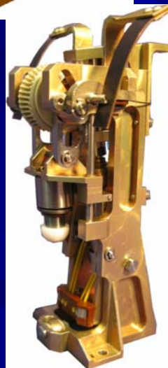
A08 Tapping Station
