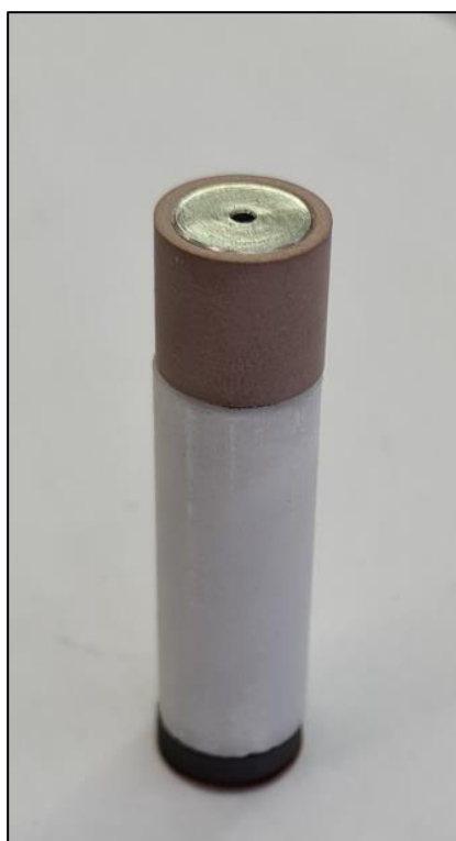
Figure 14: Components of a piston-cylinder assembly with sample capsule (top) and fully assembled assembly (bottom)
