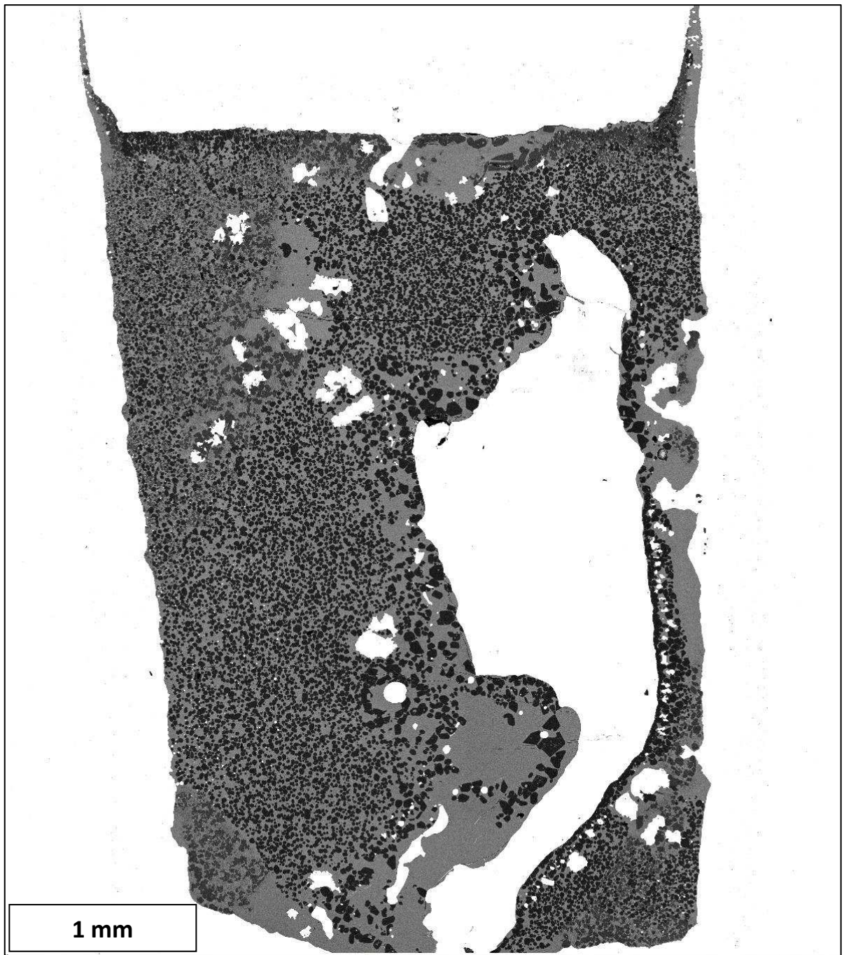
Figure 147: Overview of sample LPUM-M120-1 with capsule materials in white.
